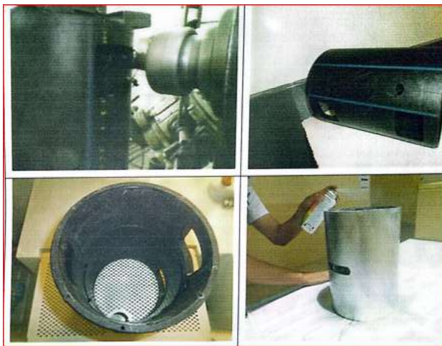
Figure 2. Machining and finishing of Pelton turbine casing
