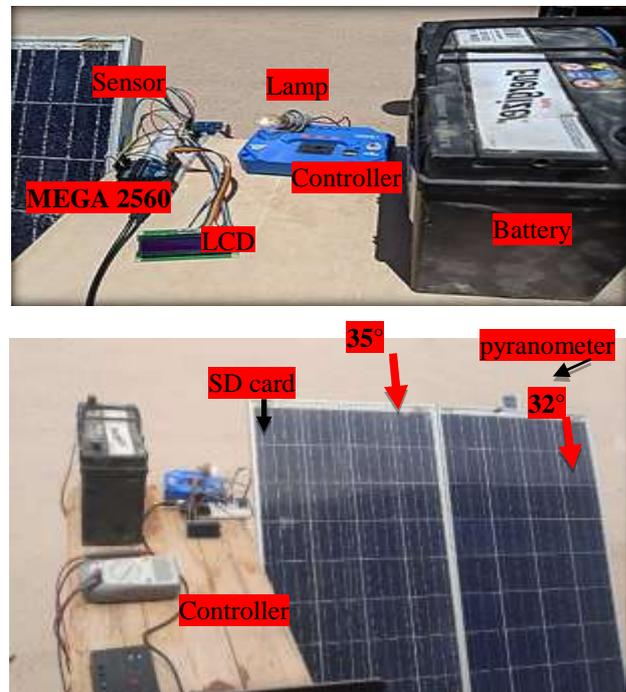
Figure 4. Experimental setup of the data logger to measure PV parameters
