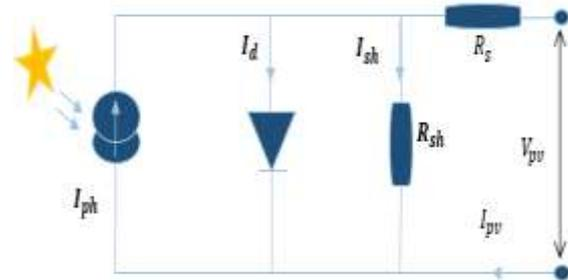
Figure.1.circuit equivalent panel solar [13]
