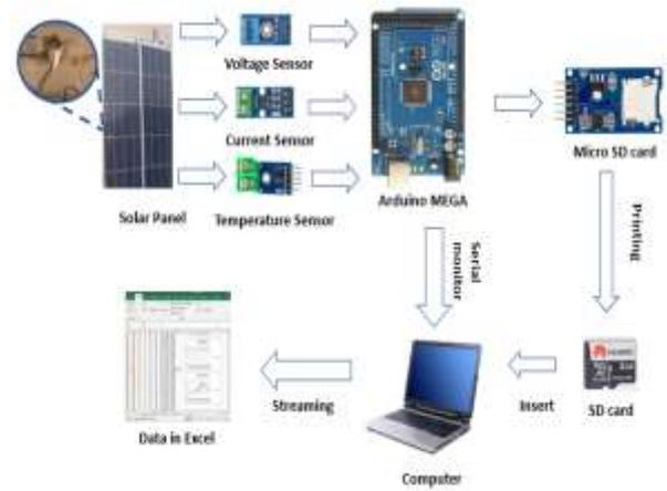
Figure.3. Real-Time Data Acquisition of Solar Panel System
