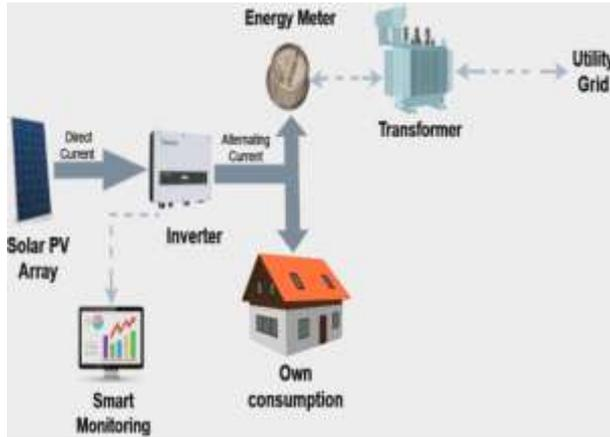
Figure 1. Grid-Connected Rooftop Solar PV System
