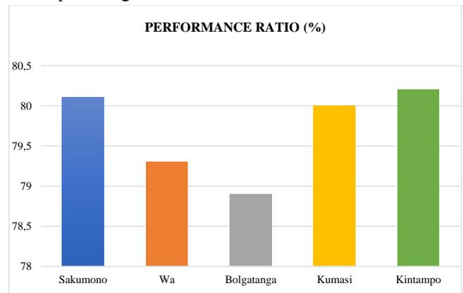
Figure 6. Performance Ratio Results from Simulation
